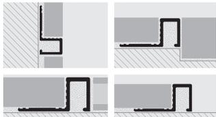
PROFINAL is a profile in natural, polished and chromed brass. It is available in three widths 8, 10 and 12.5 mm. Ideal for joining two types of floor on the same level (e.g. tile/tile or tile/wood), creating a decorative separating profile. It is also suitable as a step nosing or to create a decorative strip in the covering. It protects the edge and withstands high loads and frequent traffic.
