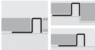
1. Choose the "PROFINAL" with the same height as the thickness of the covering. 2. Apply the adhesive onto the area of application of the profile. 3. Lay and align the profile pressing the perforated flange into the adhesive. 4. Lay the tiles, aligning them so that the top edge of the profile is "flush" with the tile. 5. Use the adhesive to seal any empty interstices.
